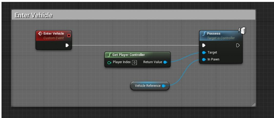
It doesn't matter from which Blueprint you call this node. The Racing Manager Blueprint also uses this node to possess the Players to the target vehicles.
